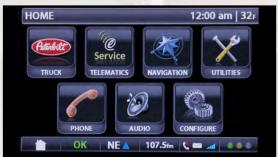
The Premium interior features the revolutionary new SmartNav<sup>TM</sup> system, an in-dash, telematics and infotainment system. SmartNav<sup>TM</sup> features a 7-inch touch screen that provides real-time vehicle monitoring, a truck-specific Garmin navigation system, hands-free Bluetooth connectivity, voice recognition, a fully integrated audio system with satellite radio as well as MP3, USB and iPod capabilities.
