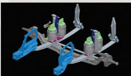
Peterbilt's proprietary Front Air Leaf Suspension is lightweight and features a 20% improvement in ride quality over taper leaf suspensions for an extremely soft ride and is compatible with air disc brakes as well as reduces tire wear. The Front Air Leaf Suspension's ride height is designed to match the popular Low Air Leaf and FlexAir rear suspensions.
