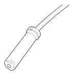
Fig. 5: Anti-lock Brake Wheel Speed Sensor
