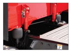
Peterbilt's Unibilt® cab sleeper system combines the cab and sleeper into a single structural unit with an independent dual air bag and shock absorber suspension for an exceptionally smooth ride.
