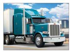
An optional Fuel Efficiency Package combines a roof fairing and trim tabs, a sleeper roof transition, a composit sunvisor, a 3-inch sleeper extender and aero mirrors to reduce vehicle drag by up to 24 percent.
