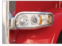
New halogen reflector, aluminum headlamps and long-life, LED directional signals are protected with an impact-resistant lens. Forward lighting is increased by 226% and bulb life by nearly 600%.
