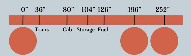
$$\begin{split} f_{Trans} &= (2500^*(196\text{-}36))/196 = 2041 \\ f_{Cab} &= (3000^*(196\text{-}80))/196 = 1776 \\ f_{Storage} &= (400^*(196\text{-}104))/196 = 188 \\ f_{Fuel} &= (1800^*(196\text{-}126))/196 = 643 \end{split}$$
