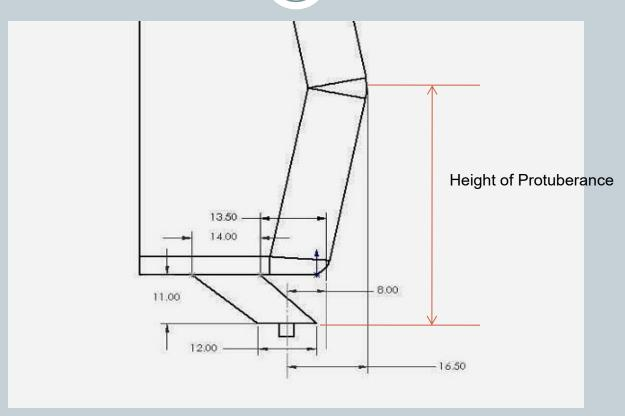
The distance from the furthest point is given by the Pythagorean equation. A<sup>2</sup>+B<sup>2</sup>=C<sup>2</sup>, A=16.5, B=51, therefore C=56.1 Always use 51 for "B"
