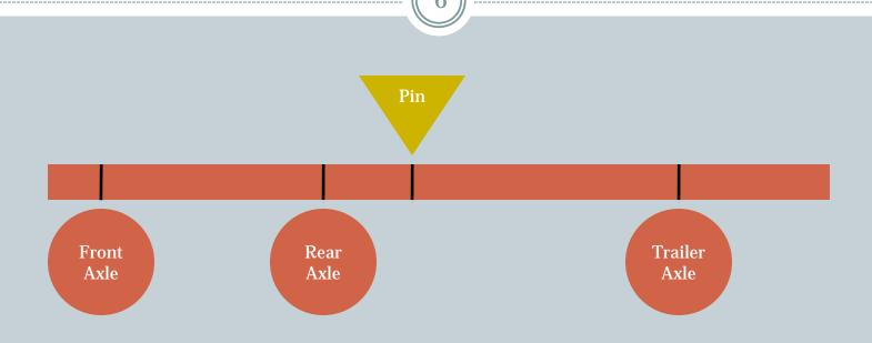
GCVW = Front Axle + Rear Axle + Trailer Axle
