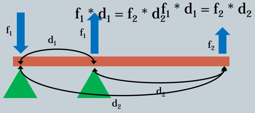
The product of force, distance pairs on a lever are equal.
