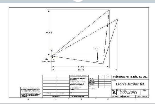
As the trailer and truck move off-angle, the cap of the trailer moves towards the truck as specified by Sin 10° \* Height of Protuberance.
