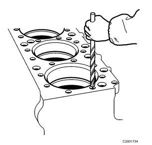
If needed, use a drill bit of the correct size. Clean out any debris from threaded holes. Turn by hand ONLY.
