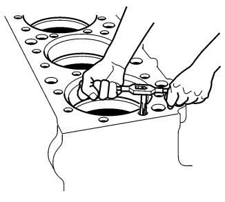
Thread the tap into the cylinder head mounting holes. Use short in and out motions to clean out threads. Continue until threads are clean, top to bottom.
