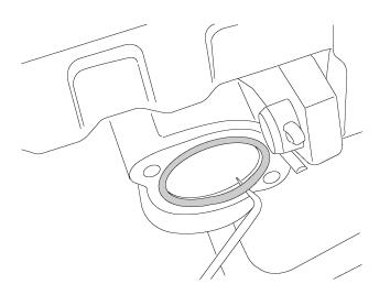
**4** Replace thermostat valve O-ring in the oil filter housing.
