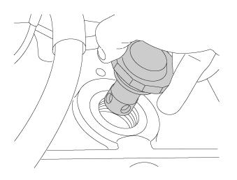
**3** Remove the cover and safety valve together as an assembly.
