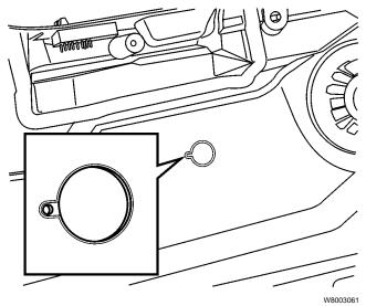
Using a 5.5 mm drill bit, drill out the area marked for crank handle, washer line-up tab.
