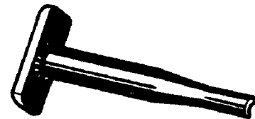
J-37451 Deutsch heavy-duty contact removal tool (Kent-Moore)
