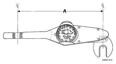
The simpler method is to place the open end of the wrench extension at a 90° angle to the torque wrench as shown above. This will not change the distance from the center of the bolt to the end of the wrench handle (A).
