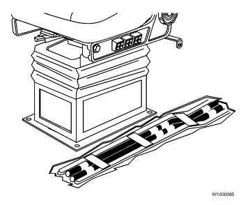
The cab electrical wiring and air tubing to the seats are routed in channels in the floor on VN & VHD cabs. The floor mat covers the wiring and tubing without any extra protection.
