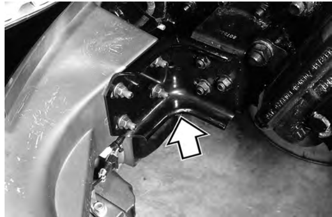
SMC bumper mounted to front bumper mounting bracket
