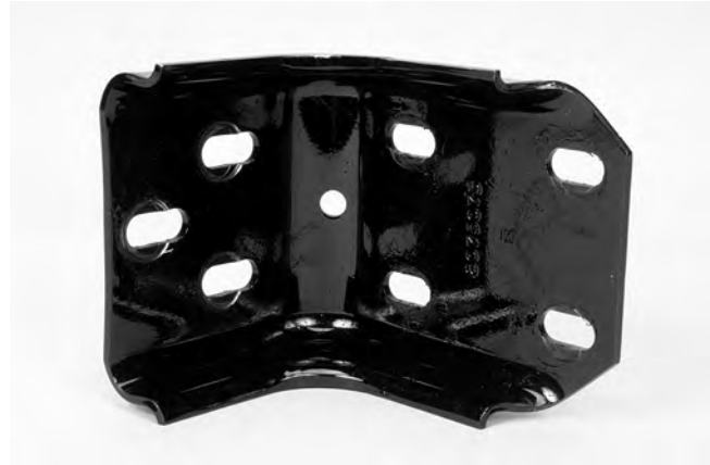
Front bumper mounting bracket for SMC bumper
